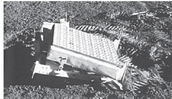
Figure 8b Array of corner reflectors left on the moon by the Apollo astronauts. A laser pulse from the earth, aimed at the reflectors, returns straight back to the laser. By measuring the time the pulse takes to go to the reflectors and back, the distance to that point on the moon and back can be accurately measured.
