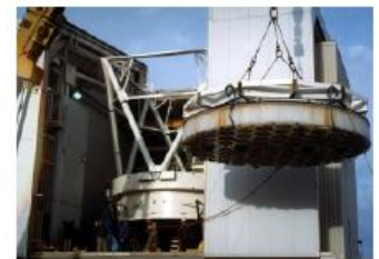
Figures 59d,e The 6.5 meter MMT telescope atop Mt. Hopkins. Above, the mirror has not been silvered yet. The blue is a temporary protective coating. Below, the mirror is being hoisted into the telescope frame.
