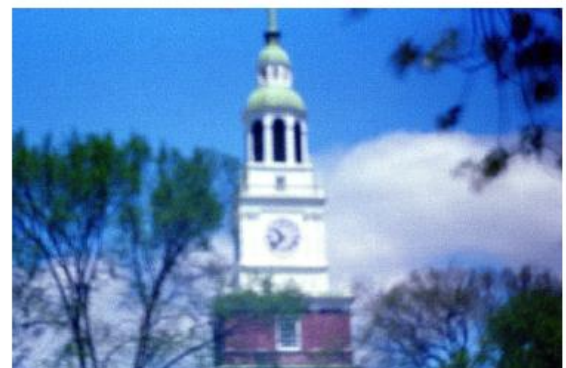
Figure 49b Photograph of Baker library tower, taken with the pinhole camera above. If we had used a smaller hole we would have gotten a sharper focus.
