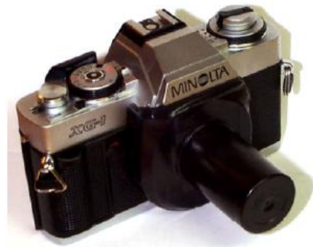
Figure 49a We made a pinhole camera by replacing the camera lens with a plastic film case that had a small hole poked into the end.
