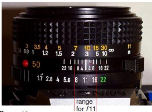
Figure 48c Camera lens. This lens is set to f11 , and adjusted to a focus of 3 meters or 10 ft. At this setting, the depth of field ranges from 2 to 5 meters.
